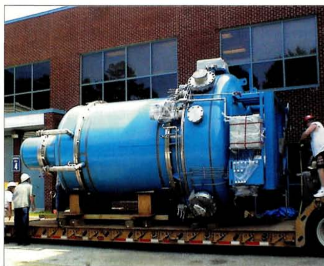
The 2 K cold box for the new Spallation Neutron Source facility at Oak Ridge is inspected prior to shipment. (D Arenius.)
