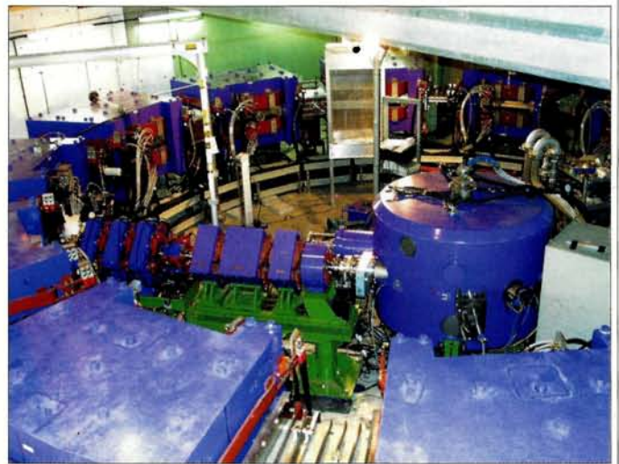
The 12-sector 150 MeV proton FFAG recently built at KEK.
