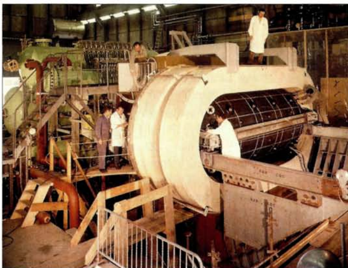
The Gargamelle heavy-liquid bubble chamber during its installation at the Proton Synchrotron in September 1970.
