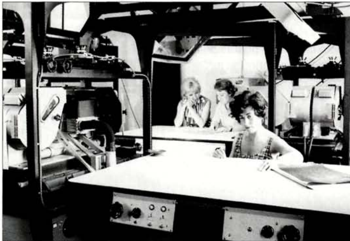
The analysis of bubble-chamber film took place both at CERN and in the collaborating institutes. This is a typical scene of scanners at work on the projection and measuring machines at CERN.
