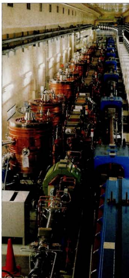
The side-by-side electron and positron rings in the KEKB collider. (Photo courtesy of KEK.)
