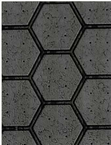
Fig. 3a. (Top, left.) The ASIC chip bonded to its ceramic package. Fig. 3b. (Bottom, left.) A close-up of the chip's honeycomb pixel matrix. Fig. 4a. (Top, centre.) The reconstructed track of a 5 keV photoelectron. Fig. 4b. (Top, right.) Track direction reconstruction algorithm: red line, first step; blue line, second step. Fig. 5. (Bottom, right.) The raw data for the event in figure 4.
